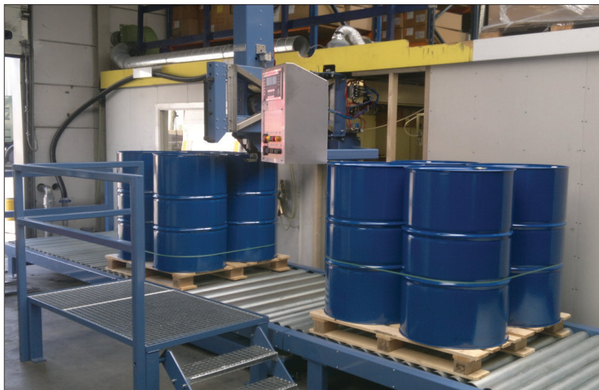
Semi-automatic pallet IBC/drum filling of foaming products by means of a sub-level filling lance.
