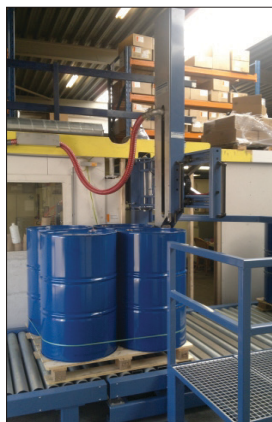
Semi-automatic pallet IBC/drum filling of foaming products by means of a sub-level filling lance.
