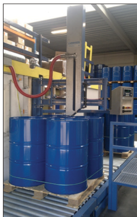
Semi-automatic pallet IBC/drum filling of foaming products by means of a sub-level filling lance.
