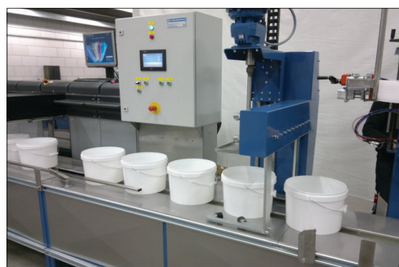
GemiFill GR-M combined with stepping type conveying system, volumetric tinting of base material, mixing unit, lid placing & closing.
