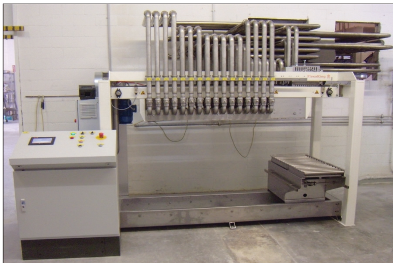
Gravimetric filling installation for 32 components by means of a moveable scale. All components connected by piping to fixed tanks and exchangeable IBC containers.
