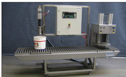
GemiFill GR-60. Explosion proof executed with non-driven roller track and lid presser.
