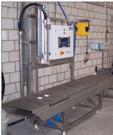
Filling of foaming products (e.g. cleaning products) by means of a sub-level filling lance.
