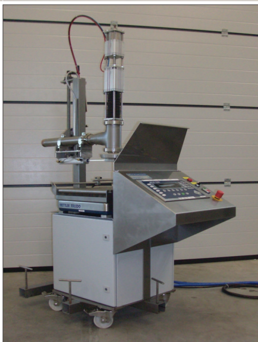
GemiFill GR-60 in basic execution. Non-explosion proof with 60 kg. scale.
