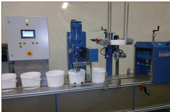
GemiFill GR-fully automatic filling line with mixer, lid placing & lid closing.
