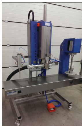
GemiFill S with nitrogen purging & lid presser.
