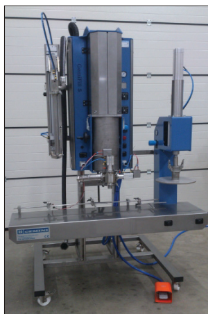
GemiFill S with filling lance & lid presser.
