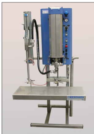
GemiFill S with sub-level filling lance.
