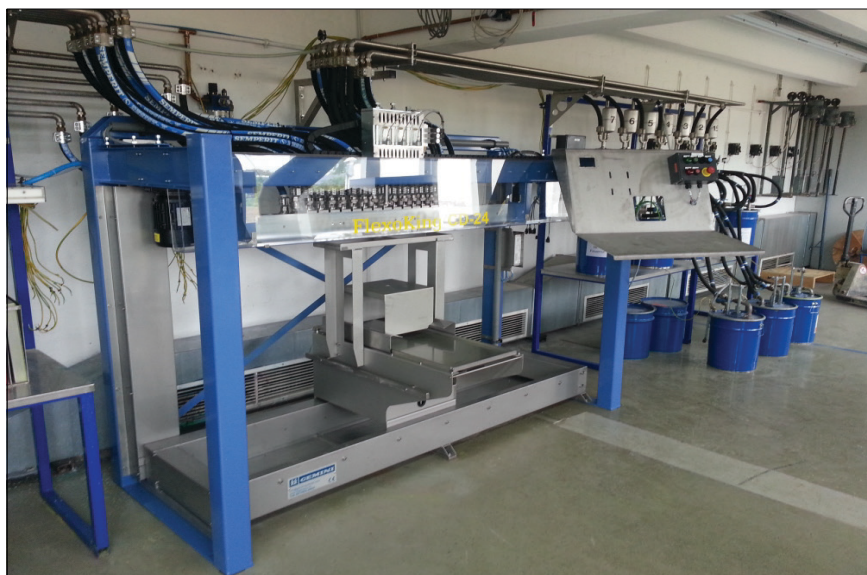
FlexoKing CD. Explosion proof executed with fixed valves and moving scale.
