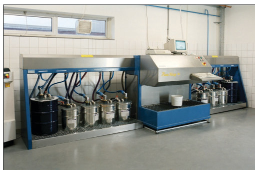
Non-explosion proof executed. Colorant drums in horizontal arrangement.
