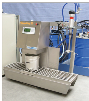
FlexoKing CD with roller track and mixer unit.
