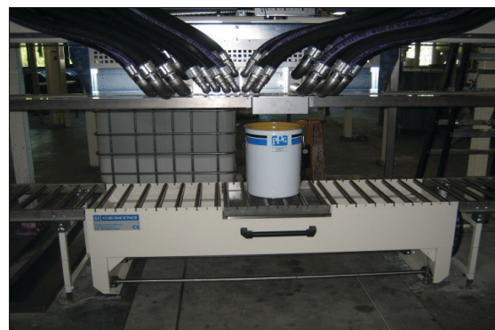
Linear dispensing head with scale integrated in roll conveyor system. Roller track can be pushed backwards for batch dispensing.
