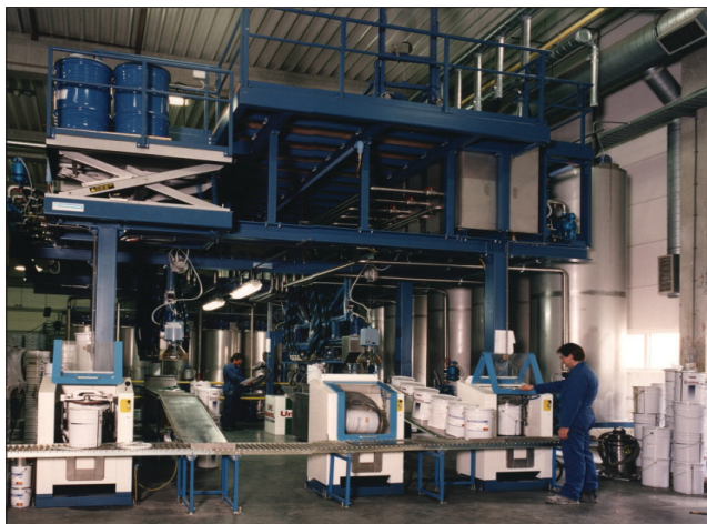
Project with 2 linear type dispensing heads for simultaneous dispensing.
