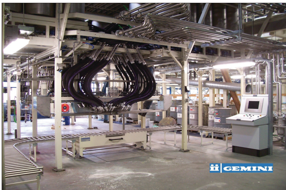
FlexoKing FT-40 for batch dispensing as well as "in-can" tinting. Explosion proof executed for Zone II.
