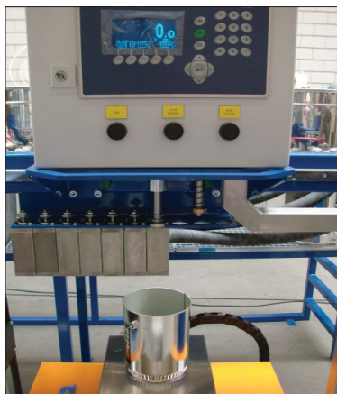
GemiTint ED-14 dispensing system. A low cost manual or semi-automatic dispenser with manual valve positioning system. The above system has 14 dispensing valves.
