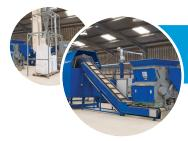
**Plastic Recycling:** we also offer full-scale plastic recycling systems - a great solution for any IBCs which are unable to be reconditioned. Systems can include grinding, separation, wash, rinse, drying, granulation, and dispensing.
